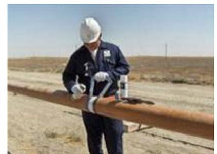
the location of the imperfection by flux leakage. In this magnetic particle testing technique, dry particles are dusted onto the surface of the test object as the item is magnetized.
